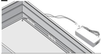
Using supplied LED layout, remove tape from module and press in place. For best illumination, install modules two-thirds of the way towards the back of the box for single sided signs and centralised for double-sided signs
