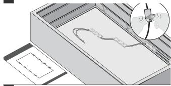
4 Drill a suitably sized hole out the back of the sign for connection to DC power supply.
