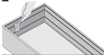
3 Secure LEDs by gluing modules in place.
