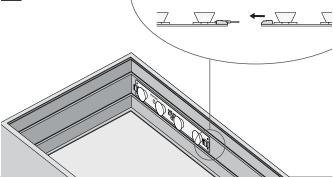
4 Using Wago connectors, wire up the LED bars to the transformer, ensuring not to exceed the maximum series. Wire in parallel if required. Exceeding the maximum series will result in voltage drop.
