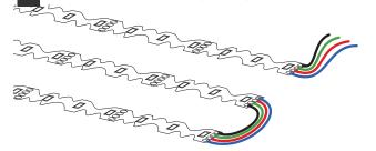
2 Ensure that your channel letter or application area is clean and free of debris. Remove adhesive liner from the back of strip and press flex strip into place.
