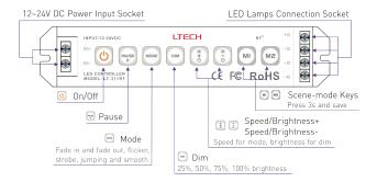
\* Press PAUSE in 3 seconds, the buzzer can be on or off.
