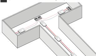
Drill holes out the back of the letters or sign box for connection to DC power supply
