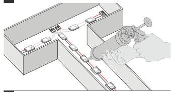
Wire the LED modules from the sign to the power supply. If there are multiple letters/signs they should be connected in parallel to eliminate voltage drop and ensure consistent brightness.
