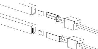
Apply silicone glue to cut end of strip, and slide end cap over. Clean up excess silicone with a clean cloth. Silicone will cure in 4 hours.
