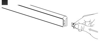
Apply silicone glue to cut end of strip, and slide cover over.
