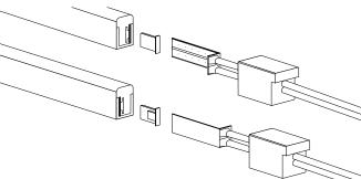
Novaneon strip can be mounted using supplied clear clips. When handling strip, take care to only bend horizontally and do not twist/stretch strip as this may damage internal components.
