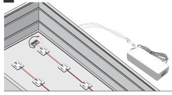
2 Using supplied LED layout, remove tape from module and press firmly into place.
