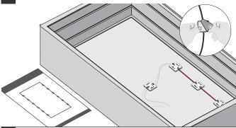
4 Drill a suitably sized hole out the back of the sign for connection to DC power supply.
