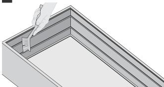
3 Secure LEDs by gluing modules in place. Ensure glue does not come into contact with LED lense as this will affect the light hue.
