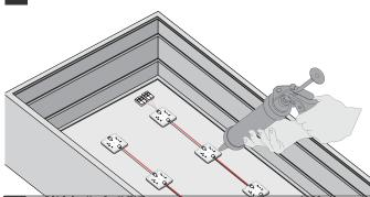
Connect modules from the sign to power supply, making sure to not exceed maximum series. Exceeding the maximum series will result in voltage drop.
