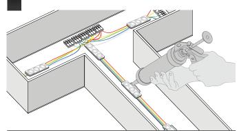
6 Connect the LED modules from the sign to the receiver and power supply. If there are multiple letters/signs, they should connected in parallel to avoid voltage drop.
