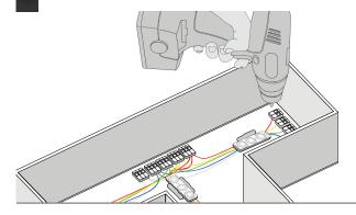
Remove tape from the rear side and stick LED modules in place using supplied LED layout.
