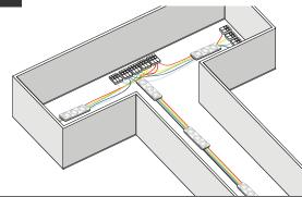
Drill holes out the back of the letters or sign box for connection to DC power supply
