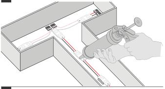
Wire the LED modules from the sign to the power supply. If there are multiple letters/signs they should be connected in parallel to eliminate voltage drop and ensure consistent brightness.
