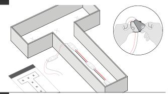
4 Secure LEDs by gluing modules in place.
