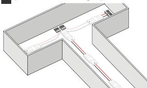
Drill holes out the back of the letters or sign box for connection to DC power supply.
