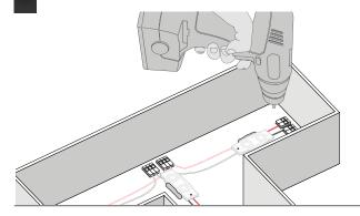
2 Using supplied LED layout, remove tape from the rear side and stick LED modules in place.
